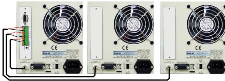
9923 is connected to three electronic loads
