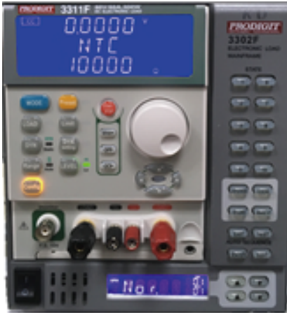
3302F frame with NTC module set NTC resistance is 10.00K \Omega
